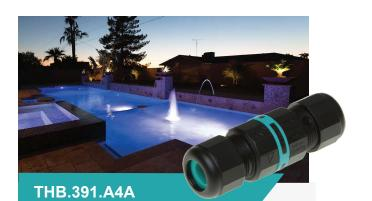
Connection: In-line Installation: Fixed connectors (re-accessible) Number of Poles: 4 Operating current: max. 32A Operating voltage: max. 450V AC Cable diameter (min-max): 7.0mm - 12mm **IP Protection: IP68**
